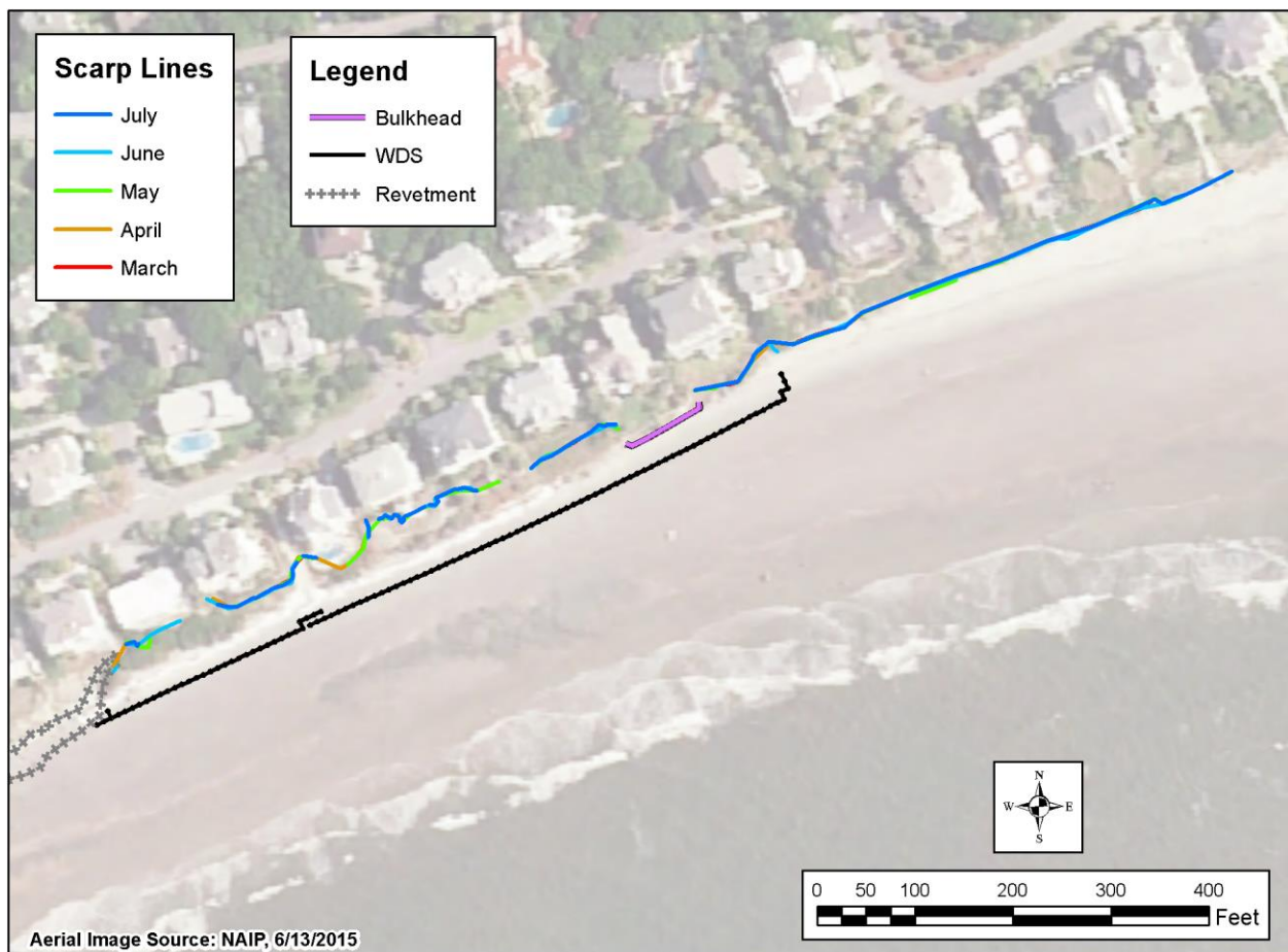
Figure 4-37. Scarp lines contours at BE
