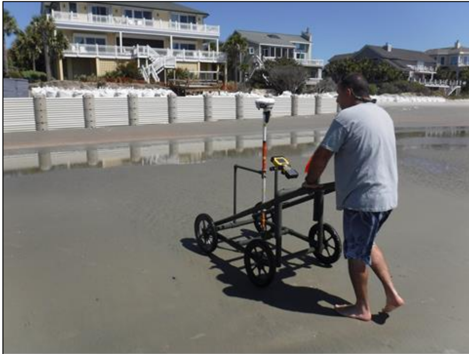
Figure 3-1. Cart used for survey of beach transects on flat beach slopes
