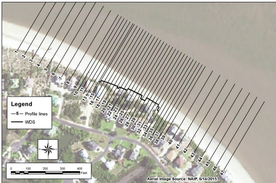
Figure 3-2. Beach profile survey transect lines at Harbor Island
