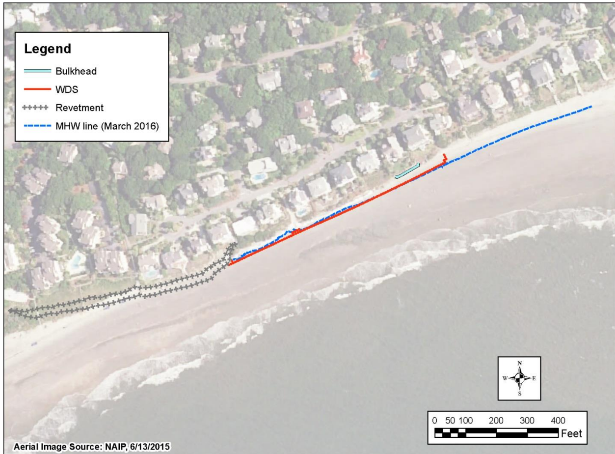
Figure 2-26. Aerial view of eroding shoreline segment and WDS location at Beachwood East
